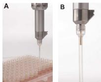
3. Aspirate sample into Neon™ Pipette
