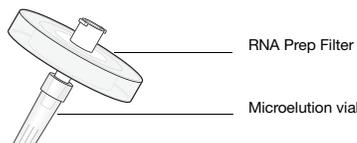
16 Add 1 µL of RNase Inhibitor (PN N8080119) to 100 µL of RNA elution solution and add solution to the tip of the RNA filter.
