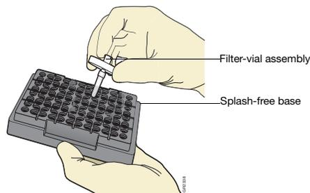
18 When the spin is finished, repeat steps 15–16 with the same eluate to ensure that all RNA is removed from the RNA prep filter.
