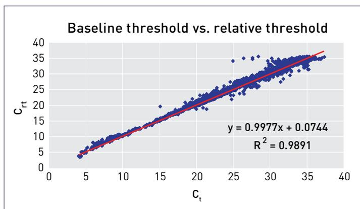
Figure 2.  $C_{rt}$  is strongly correlated to  $C_t$ . A total of 7,710 individual TaqMan® Assays with a wide range of  $C_q$  values (5–35) were run on the OpenArray® platform.  $C_{rt}$  and  $C_t$  values were generated for each through-hole, and strong correlation ( $R^2 = 0.9891$ ) was observed for the two methodologies.
