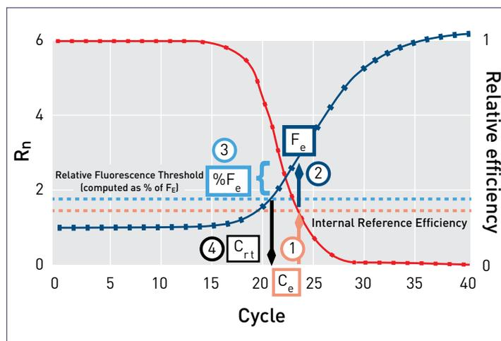
**Figure 5. The relative threshold ( $C_{rt}$ ) method.** The figure and steps below describe how the  $C_{rt}$  is calculated. The amplification curve is in blue; the model of the reaction efficiency curve is in red; the y-axis on the left goes with the blue amplification curve, and the y-axis on the right goes with the red curve.  $C_{rt}$  is determined in four steps:
