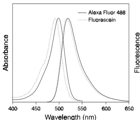
**Figure 1.** Normalized absorption and fluorescence emission spectra of Alexa Fluor 488 and fluorescein goat anti-mouse IgG conjugates.
