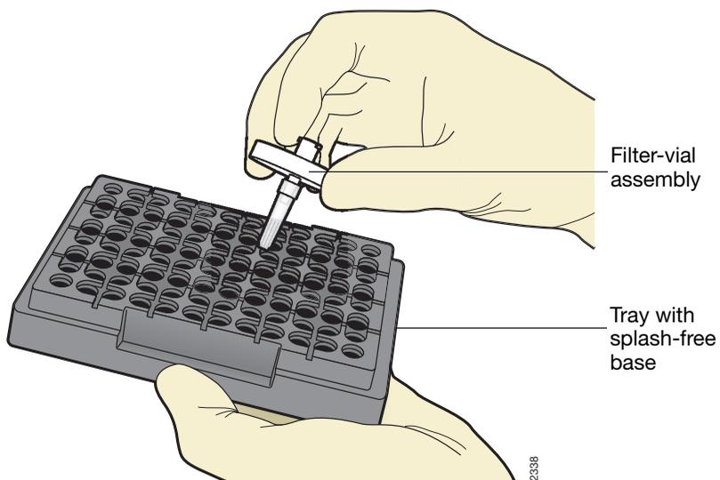
**Figure 4-3 Filter-vial-base assembly**
