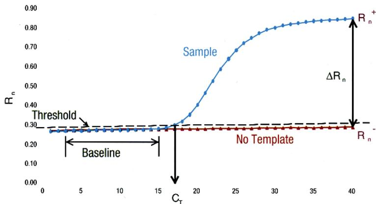
Figure A-1 Model of a single amplification plot, showing terms commonly used in quantitative analysis
