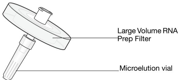
**Figure 4-2 Filter-vial assembly**
