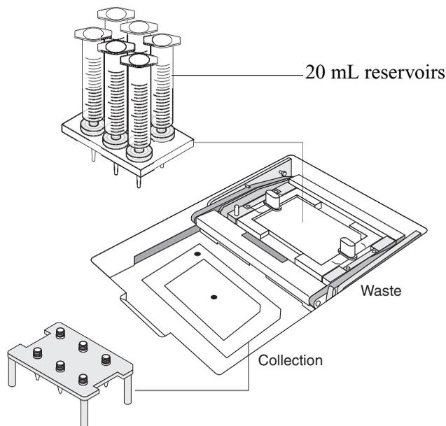
Load the assembled 2-mL Tube Collection Plate right before moving the carriage over to the collection position.
