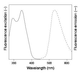
Figure 3. The normalized excitation and emission spectra of the ELF 97 alcohol precipitate, which is generated by enzymatic cleavage of the soluble ELF 97 phosphatase substrate.
