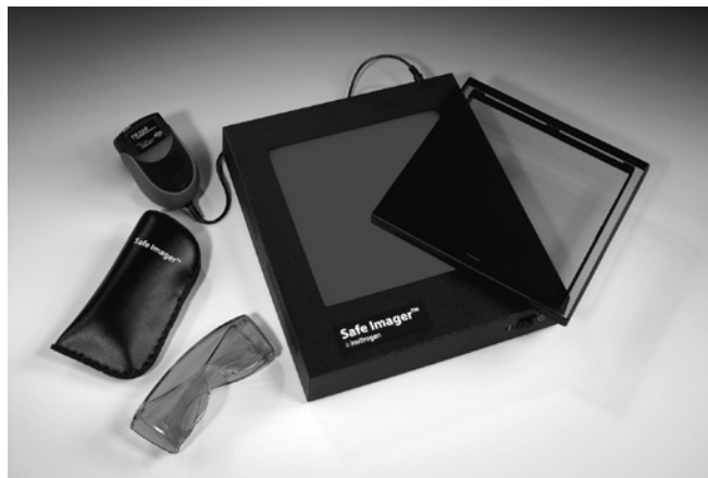
Figure 1. The Safe Imager™ blue-light transilluminator.
