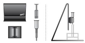
Attach MidiMACS<sup>™</sup> Separator or QuadroMACS<sup>™</sup> Separator to the MultiStand and place LS Column in the separator. Place a collection tube under the LS Column.
