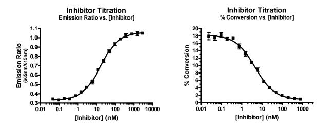
The inhibition of DAPK1 with Staurosporine is displayed above. The inhibition curve is plotted as both Emission ratio versus inhibitor concentration and % conversion versus inhibitor concentration (See Appendix C) for comparison.
