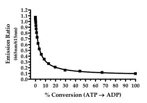
(C.2) Fit the plot to a 3-parameter hyperbolic model using an appropriate data analysis program. The following equation can be used with GraphPad<sup>™</sup> Prism<sup>®</sup> software:
