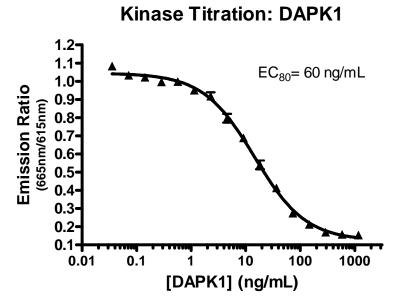
Representative data of the titration of DAPK1 is shown above. Although assay window and signal will vary between plate readers, the quality of the data generated should be comparable to the data presented above. For inhibitor titration experiments, the amount of kinase required to observed an  $\sim 80\%$  decrease in the assay window (the EC80) is determined. From the example data above, 60 ng/mL (0.8 nM) of kinase was required to achieve the 80% decrease in the assay window.
