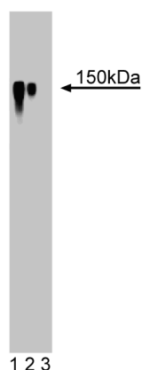
Western blot analysis of Btf on a Jurkat cell lysate (Human T-cell leukemia; ATCC TIB-152). Lane 1: 1:250, lane 2: 1:500, lane 3: 1:1000 dilution of the mouse anti-human Btf antibody.
