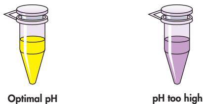
Figure 3 Indicator dye in solubilization and binding Buffers PBI, QG, and ERC identifies optimal pH for DNA binding.
