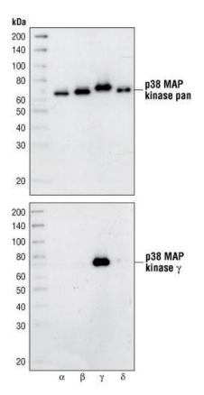
Western blot analysis of purified recombinant full-length p38 MAPK GST fusion protein, using p38 MAP kinase pan antibody (upper) or p387 MAPK Antibody (lower).
