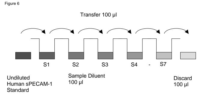
In case of an <u>external standard dilution</u> (see 9.4.1), pipette 100  $\mu$ l of these standard dilutions (S1 - S7) in the standard wells according to Table 1.
