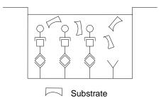
A coloured product is formed in proportion to the amount of human TNF- $\alpha$  present in the sample or standard. The reaction is terminated by addition of acid and absorbance is measured at 450 nm. A standard curve is prepared from 7 human TNF- $\alpha$  standard dilutions and human TNF- $\alpha$  sample concentration determined.
