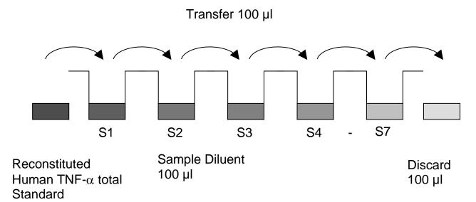
In case of an <u>external standard dilution</u> (see 9.5.1), pipette 100  $\mu$ l of these standard dilutions (S1 - S7) in the standard wells according to Table 1.
