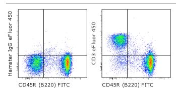
Staining of C57Bl/6 splenocytes with Anti-Human/Mouse CD45R (B220) FITC (cat. 11-0452) and 0.5 ug of Armenian Hamster IgG Isotype Control eFluor® 450 (cat. 48-4888) (left) or 0.5 ug of Anti-Mouse CD3e eFluor® 450 (right). Total viable cells were used for analysis.
