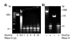
ShortCut RNase III digestion of dsRNA: (A) Varying amounts of ShortCut RNase III were incubated with 2 µg of a 500 bp dsRNA for 20 minutes at 37°C in a 50 µl reaction. Digests were analyzed by 20% TBE polyacrylamide electrophoresis. Marker lane contains a mixture of 21 bp siRNA Marker and 100 bp DNA Ladder (NEB #N3231). (B) dsRNA fragments (1 kb and 175 bp) were digested with ShortCut RNase III. Digests were analyzed by 20% TBE polyacrylamide gel electrophoresis.
