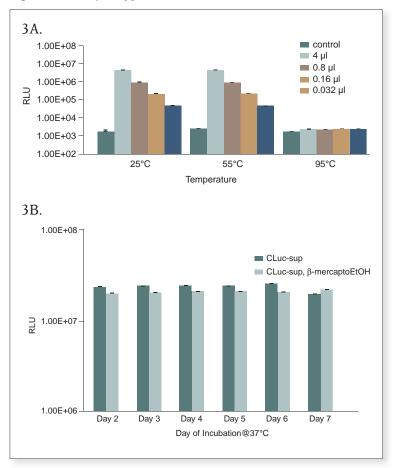
A) Supernatant obtained from stable CLuc-expressing cells was incubated at 55°C or 95°C for 30 minutes and allowed to cool to room temperature (25°C). Five-fold serial dilutions of supernatant were assayed for CLuc activity. The control is the supernatant of the parental cells from which the stable cell line was created. (B) Supernatants from stable CLuc-expressing cells, grown in medium with or without  $\beta$ -mercaptoethanol, were incubated at 37°C and assayed each day for 7 days.
