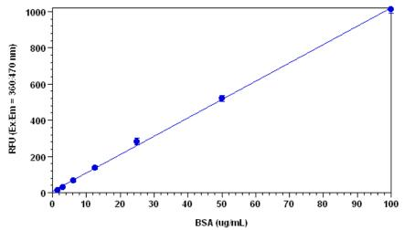
**Figure 1**. BSA dose response was measured on a 96-well back plate with the Amplite<sup>TM</sup> Fluoremetric Fluorescamine Protein Quantitation Assay Kit. As low as 0.3 μg/mL of BSA can be detected with 5 minutes incubation time (n=3).
