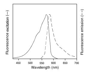
Figure 1. Normalized excitation and emission spectra of resorufin, the product of the Amplex® Red reaction.
