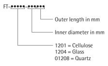
Example: FT-1201-033080 1201= Cellulose 033 = 33 mm inner diameter 080 = 80 mm outer length
